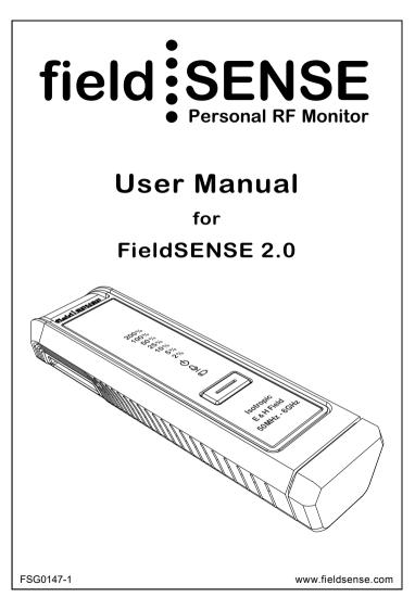
The FieldSENSE 2.0 is the next generation in Personal RF Monitors specifically designed for protecting personnel working near broadcast and telecommunications transmitting antennas from EMF/RF overexposure.
